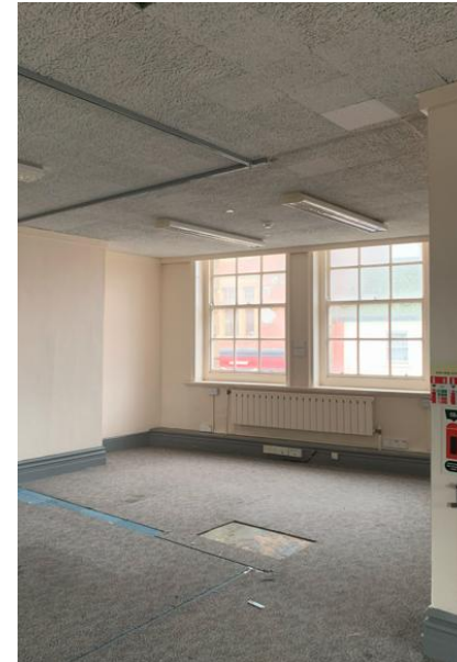
Figure 17 Change to room layout to north of the building, with evidence of wall removal, dropped ceilings and modern lighting/radiators and pipework.
